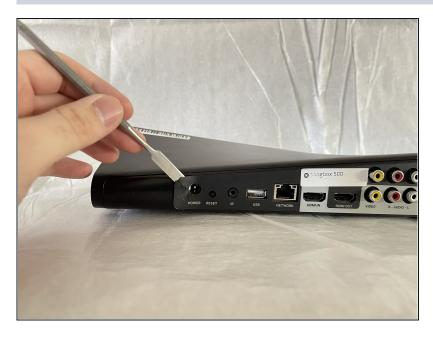
Remove the sticker on the back of the Slingbox that covers the rear screws using a spudger.
