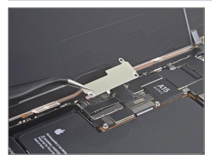
• Remove the battery connector cover.
