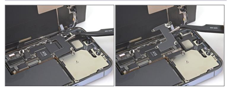
• Remove the front sensor connector cover.
