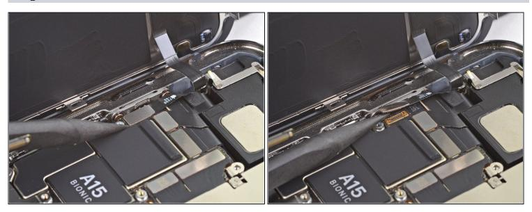
• Use the pointed end of a spudger to disconnect the front sensor assembly cable connector.
