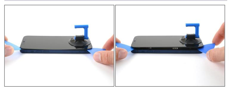
The cables along the left edge are **very easy to damage with a pick**. Follow this alternate procedure to separate the left adhesive.
