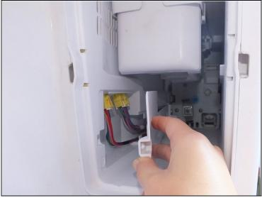
• Unscrew the 0.05 mm screw on the left side panel inside the icebox with a Phillips #0 screwdriver.
