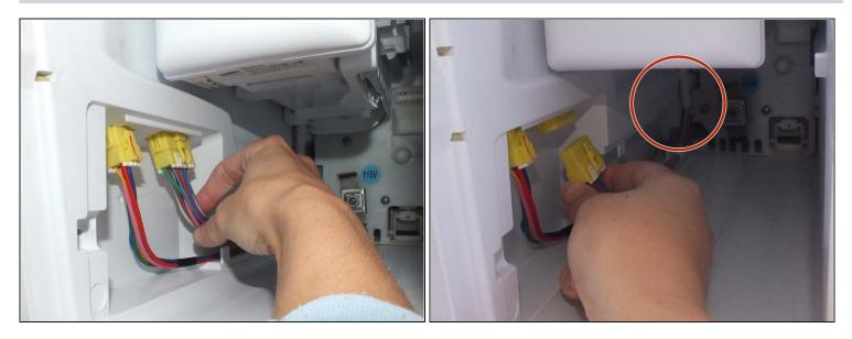
• Carefully detach the plug connected to the thick white tube located to the left in the back of the icebox.
