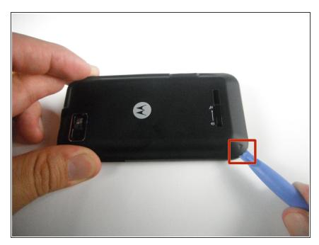
Wedge the plastic opening tool in between the back cover and the body of the phone in the opening denoted by the arrow.
