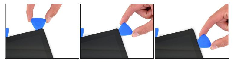
• Round the left corner with the opening pick and slide it along the top edge of the Surface. Stop when the pick is 2.75 inches (70 mm) away from the left edge.
