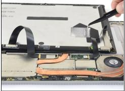
• Use your tweezers to remove the two EMI shields covering the display cable connectors.
