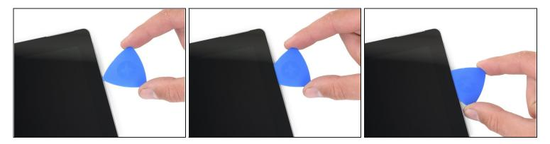
⚠ Fragile antenna cables lie under the top edge of the screen. Carefully follow the procedure to avoid damaging them.
