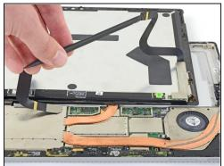
• Pry up with the flat end of a spudger to disconnect each display cable from the motherboard.
