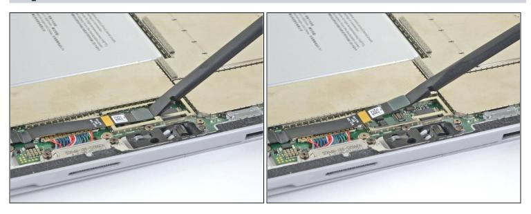
Use the flat end of your spudger to lift the microSD card reader's connector straight up out of its socket.
