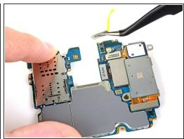
• Use a pair of tweezers to remove the small piece of tape covering the middle camera connector.
