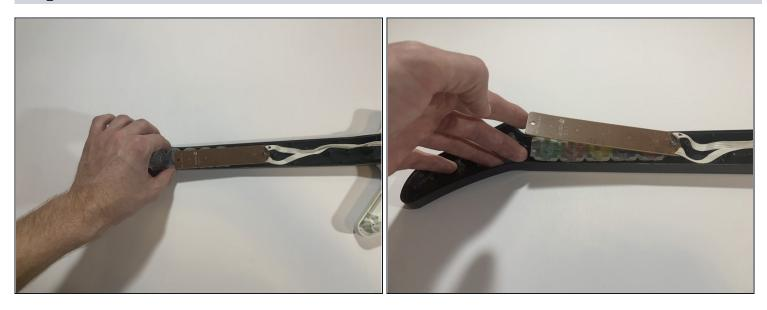
• Using your hands, insert the replacement strip underneath the key sensor board.
