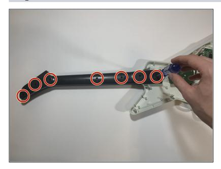
Remove all seven 12mm screws on the neck of the controller using the Phillips #2 screwdriver.
