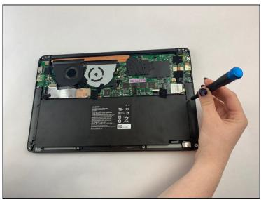
• Use a Phillips screwdriver to remove the six screws securing the battery.
