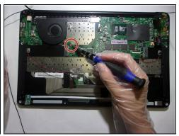
• Remove the 3.4 mm screws on the perimeter of the motherboard using a T4 Torx screwdriver.
