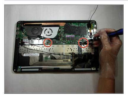
Remove the red and black cables that are attached to the motherboard.
