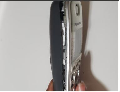
Take an opening tool or pick and slide it in between the back and front cover all the way around the phone, then pull the back case off.
