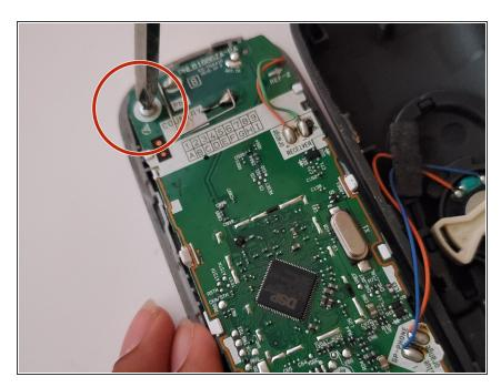
Use a Phillips #00 screwdriver to remove one 6.4 mm screw from the top left corner of the phone.
