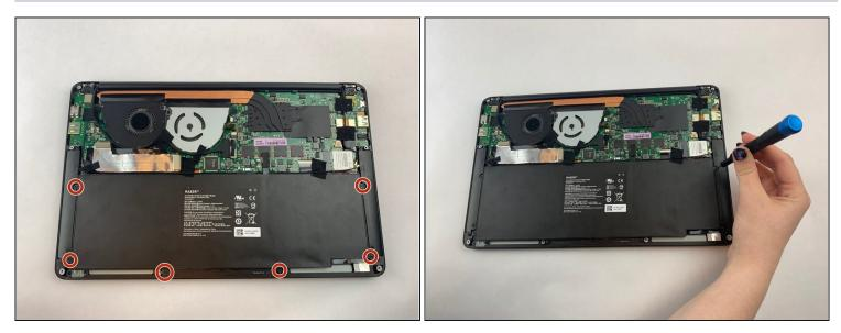
• Use a Phillips screwdriver to remove the six screws securing the battery.
