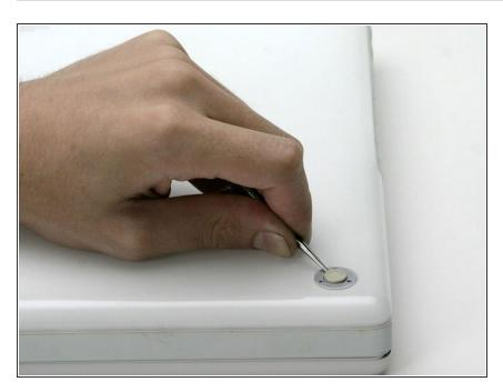
Use a pin to remove the three rubber feet from the lower case.
