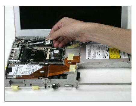
Slide the modem out of the computer, being careful to avoid catching the black plastic shielding on the surrounding cables.
