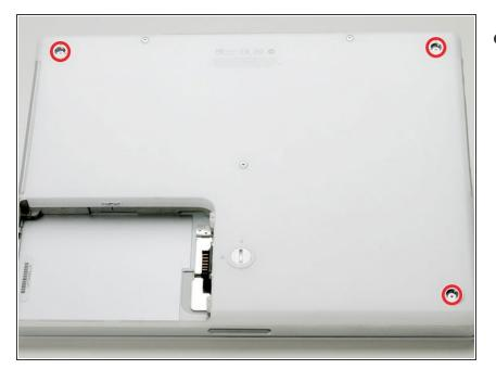
Remove the three newly-revealed Phillips screws.
