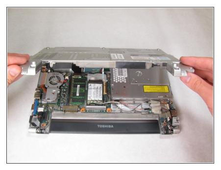
Pull up on the back casing and remove it.
