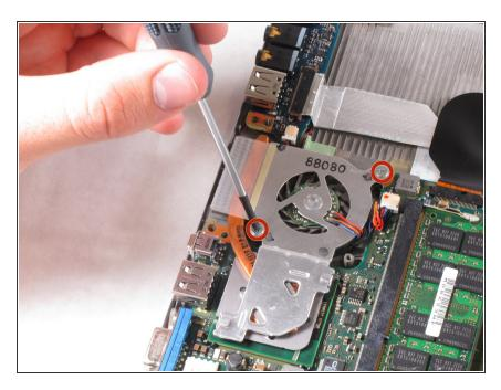
Remove the two 5.5 mm screws from the fan with the Phillips 00 screwdriver.
