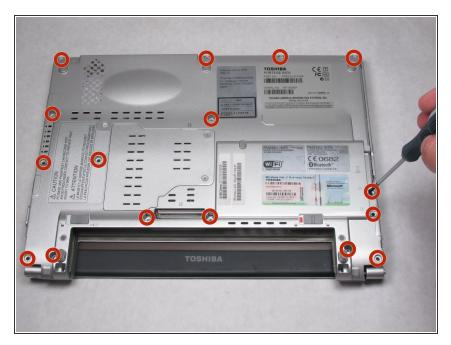
Remove the sixteen screws at the locations shown with the Phillips 00 screwdriver.
