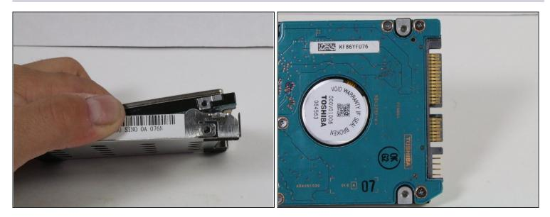
• Carefully separate the actual hard drive from the hard drive assembly.
