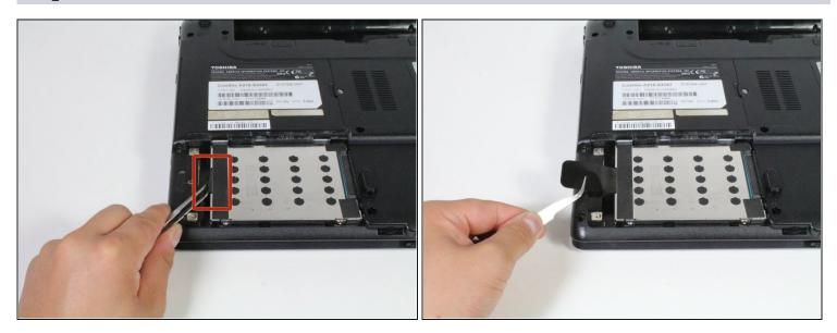
• Use a pair of metal <u>tweezers</u> to grab the plastic pull-tab that is tucked in underneath the hard drive.
