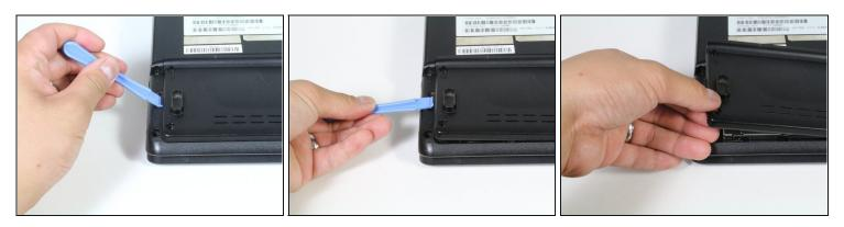
• Using a plastic opening tool, open the compartment and remove the compartment cover.
