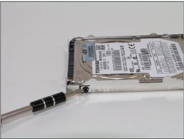
• Flip over the hard drive assembly and remove two 4mm Phillips #1 screws at the top left and right side of the hard drive housing.
