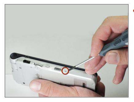
• Unscrew the 2.5mm screw located on the left side of the device with a Phillips #00 screwdriver.
