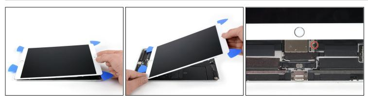
• Lift the display assembly from its top edge and carefully slide it up (towards the frontfacing camera and headphone jack), until the screw that secures the battery power connector is revealed at the bottom.
