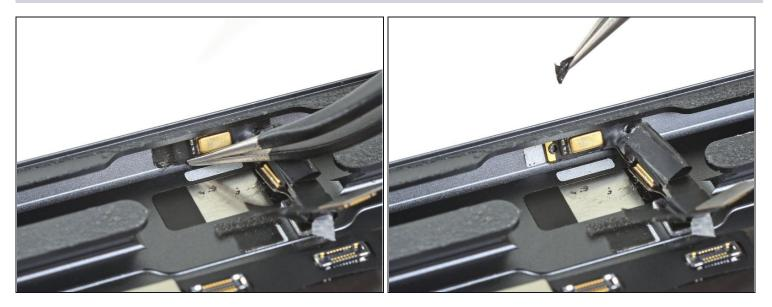
• Use a pair of tweezers to remove the small strip of tape underneath the upper lip of the rear case.
