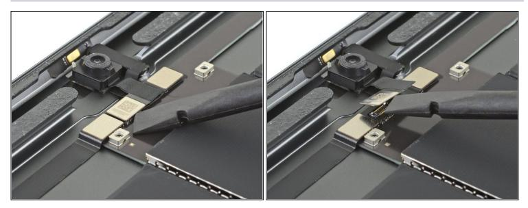
• Use the flat end of a spudger to disconnect the front camera cable by lifting straight up on the press connector.
