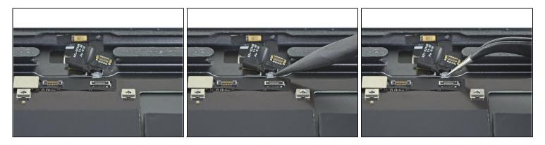
If you encounter a ball of adhesive resembling hot glue holding down the microphone assembly, use the pointed end of a spudger to pick it off.
