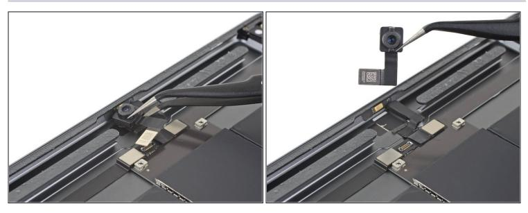
• Use a pair of tweezers to remove the front camera.
