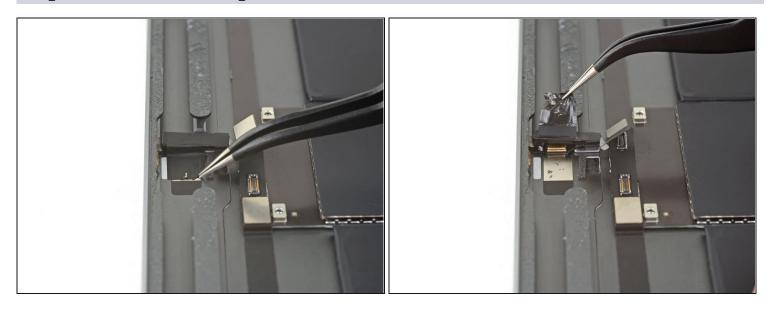
• Use a pair of tweezers to remove the tape securing the microphone assembly to the rear case.
