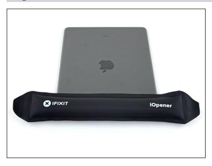
• Apply a heated iOpener to the top edge of the iPad to loosen the microphone assembly adhesive.
