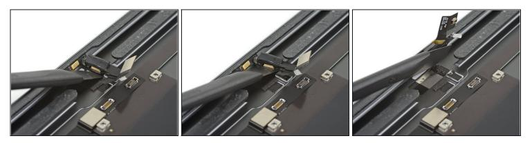
• Insert an opening pick or a halberd spudger underneath the lower microphone and peel it up from the rear case.
