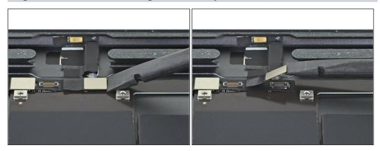
• Use the flat end of a spudger to disconnect the microphone assembly cable by lifting straight up on the press connector.
