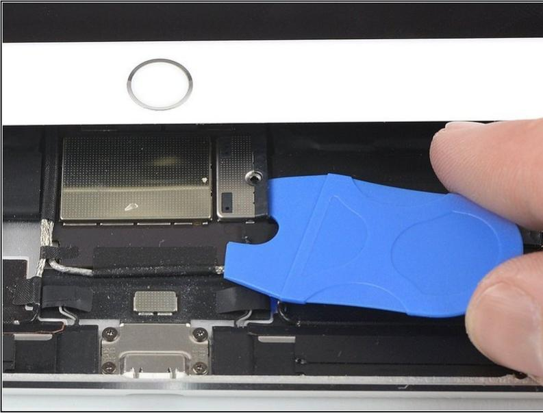
**⚠** Be careful when you isolate the battery using a battery blocker. The battery contacts are easily bent or broken, resulting in irreversible damage.
