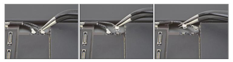
• Use a pair of <u>tweezers</u> to disconnect a logic board antenna cable by <u>lifting up on the</u> <u>cable as close to the connector as possible</u>.
