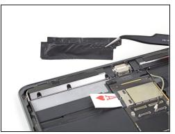
• Use a pair of tweezers to remove the tape covering the right speaker screws.
