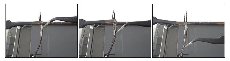
• Use a pair of tweezers to unwrap the tape securing the two antenna cables together.
