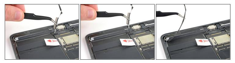
• Continue to peel the right antenna cable away from the rear case.
