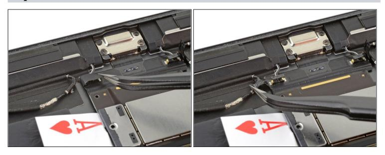
• Use a pair of tweezers to remove the tape from the back of the speaker connector.
