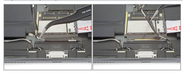
• Use a pair of <u>tweezers</u> to peel the right antenna cable away from the logic board.
