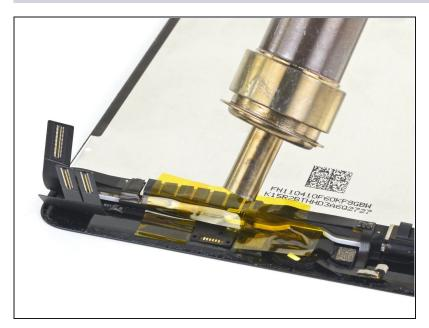
• Use a soldering iron or hot air gun to apply heat evenly to the six magnetic sensor solder pads.
