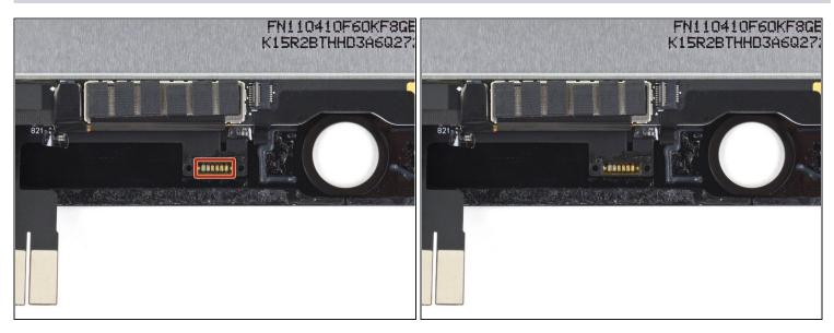
• In the next steps, you'll desolder the six solder pads securing the magnetic sensor to the screen.
