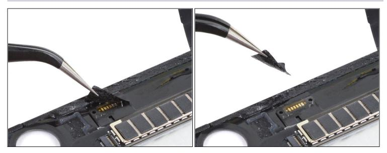
• Use a pair of <u>tweezers</u> to remove the sticker covering the magnetic sensor solder pads.
