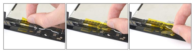
• Apply polyimide tape to the area around the magnetic sensor solder pads to protect the components from heat.
