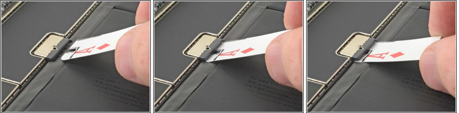
**⚠ Be extremely slow and careful when you isolate the battery using a battery blocker. The battery contacts are easily bent or broken, resulting in irreversible damage.**
