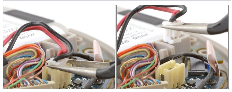
• Use a pair of tweezers to grip the edges of the battery connector, and pull up to disconnect it from the main board.
