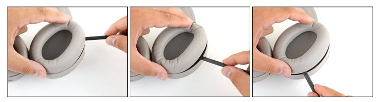
• Repeat the previous step around the perimeter of the ear cup to disconnect the remaining clips.
