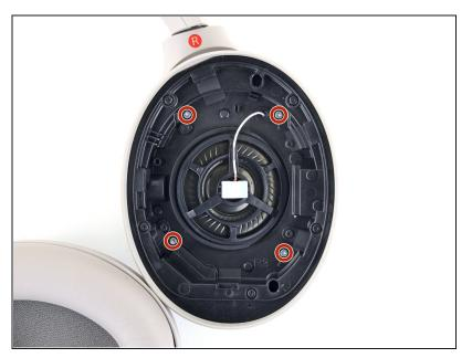
Use a Phillips screwdriver to remove the four 8.4 mm screws securing the right ear cup cover.
