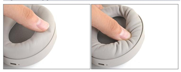
• Use your thumb to depress the **RIGHT** ear pad near the long outer edge, creating a gap between the cushion and the frame.
