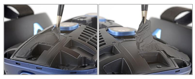
Gently peel up the stickers on either side of the front of the Vive. If possible, keep the stickers intact and reuse them.
