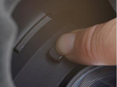
Use your finger to push the sliding faceplate release switch, sitting to the left of the lenses, toward the bottom of the Vive.
