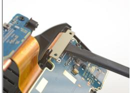
Use the flat end of a spudger to pry the LCD connectors straight up and out of their sockets on the daughterboard.
