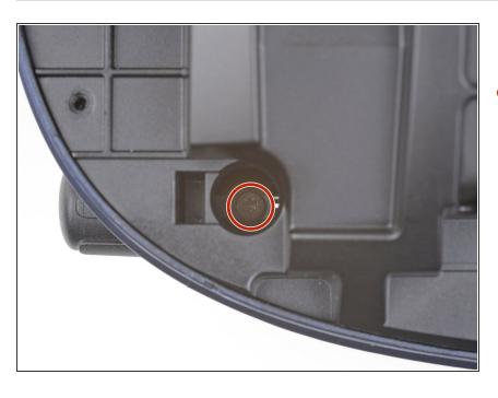
Use a T5 Torx driver to remove the 4.1 mm long screw securing the focus knob.
