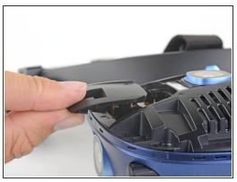
Slide the camera connector covers on either side of the LCD and motherboard assembly away from the center off of the assembly and remove them.
