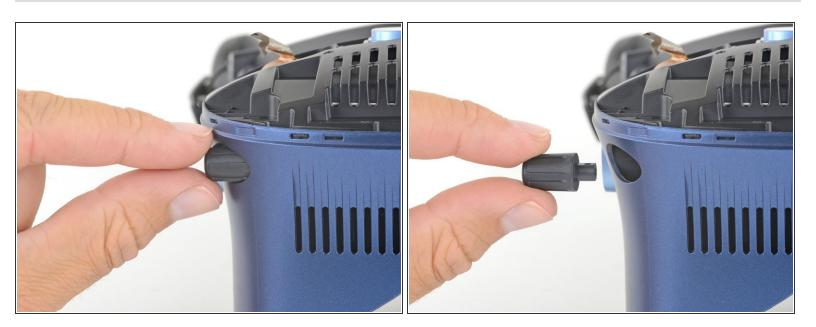
Slide the focus knob out of the plastic housing, off of the focus rod, and remove it.
