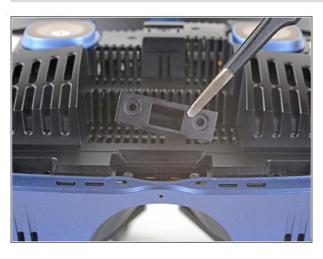
Remove the microphone cover from the bottom edge of the headset.
