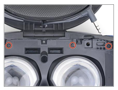
Use a T5 Torx driver to remove the three 4.1 mm long screws securing the LCD and motherboard assembly.
