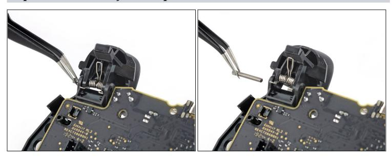
• Use a pair of <u>tweezers</u> to pull the cylindrical pin from its guide.
