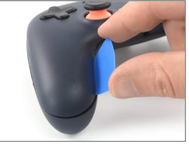
• Insert an opening pick in a steep angle into the gap you created to prevent the first clamp from popping back into its closed position.
