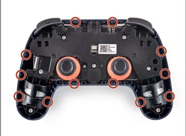
• The front cover assembly of the Stadia controller is held in place by various tight plastic clamps. They are very hard to open and snap back in place easily.
