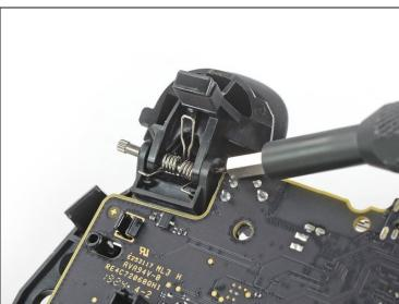
Use a SIM eject bit to push against the inner end of the cylindrical pin holding the left trigger in place.
