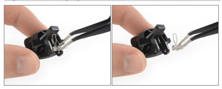
• Use a pair of tweezers to remove the spring from the right trigger.
