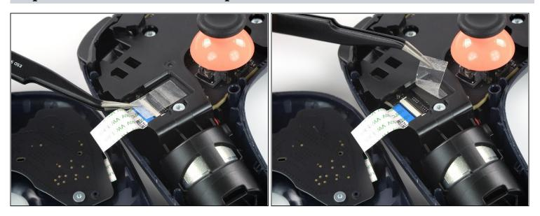
• Use a pair of <u>tweezers</u> to peel the clear protective tape off the ZIF connector on the left side of the rear case.
