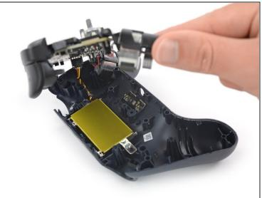
• Carefully lift the left edge of the motherboard assembly in order to access the battery connector.
