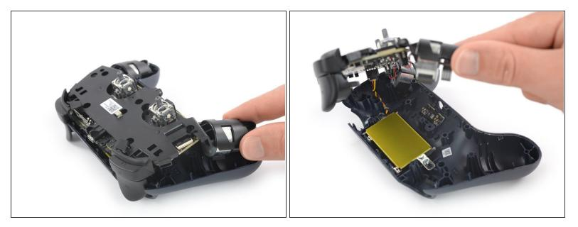
• Carefully lift the left edge of the motherboard assembly in order to access the battery connector.
