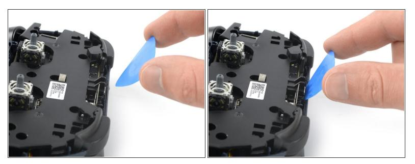
Insert an opening pick at the top edge of the Stadia controller to prevent the charging port from snapping back into place.
