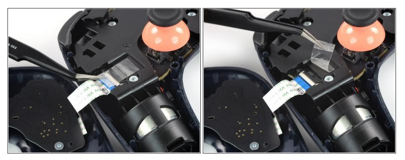
Use a pair of tweezers to peel the clear protective tape off the ZIF connector on the left side of the rear case.
