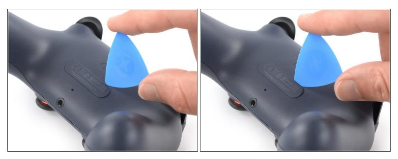
Insert the tip of an opening pick into the gap between the plastic screw cover and the rear case of the controller.
