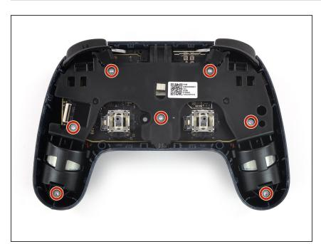
Use a Torx T8 screwdriver to remove the seven 9.6 mm-long screws securing the motherboard assembly.
