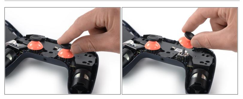
Use your fingers to remove the right thumbstick by pulling it upwards and off the right joystick.
