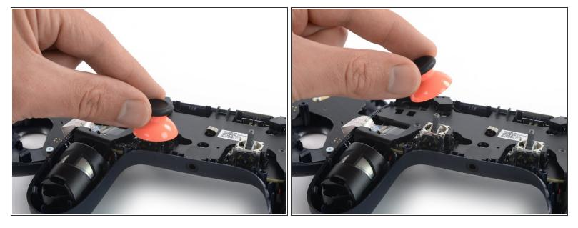
• Use your fingers to remove the left thumbstick by pulling it upwards and off the left joystick.
