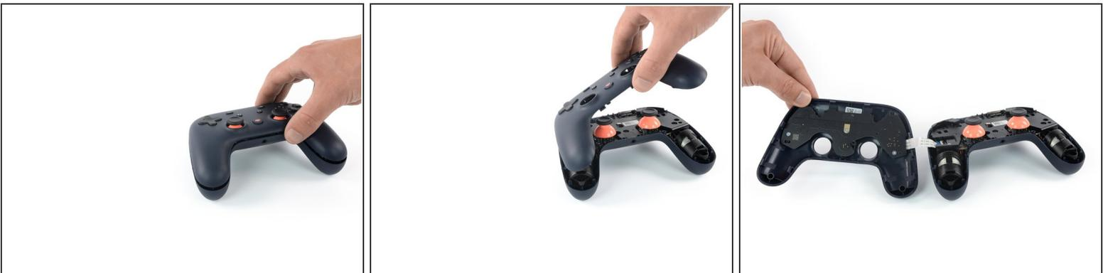
**⚠ Avoid straining the front cover assembly cable during this step.**
