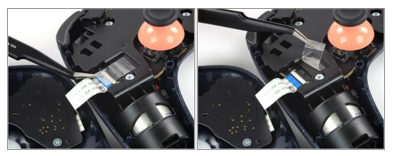
Use a pair of tweezers to peel the clear protective tape off the ZIF connector on the left side of the rear case.
