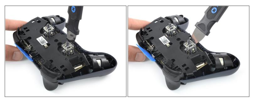
• Pry up the motherboard assembly by tilting the Jimmy downwards.
