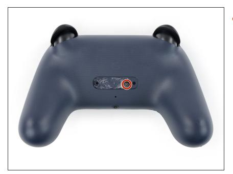
Use a Torx T8 screwdriver to remove the 9.6 mm-long screw securing the rear case.
