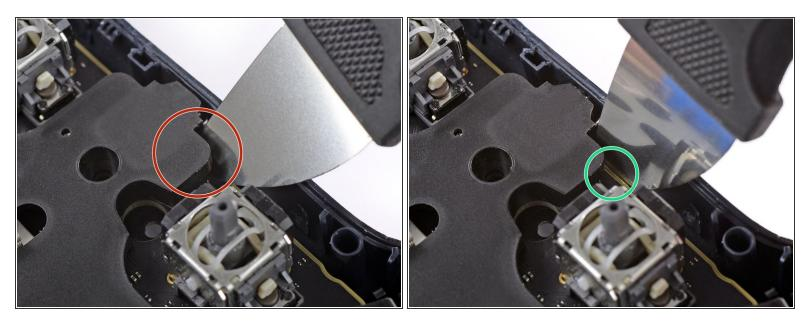
In the following step you'll free the headphone jack from its recess in the controller housing:
