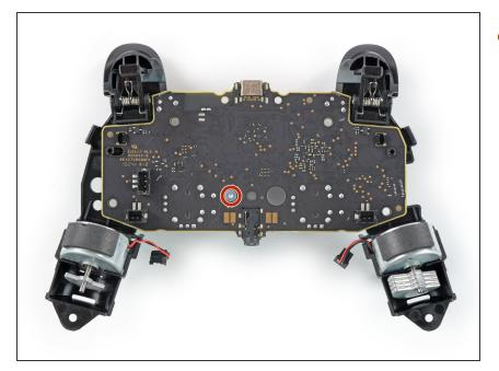
Use a T6 Torx screwdriver to remove the single 6.1 mm-long screw securing the motherboard.
