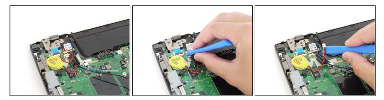
• Using the plastic opening tool, disconnect the CMOS battery from the motherboard.
