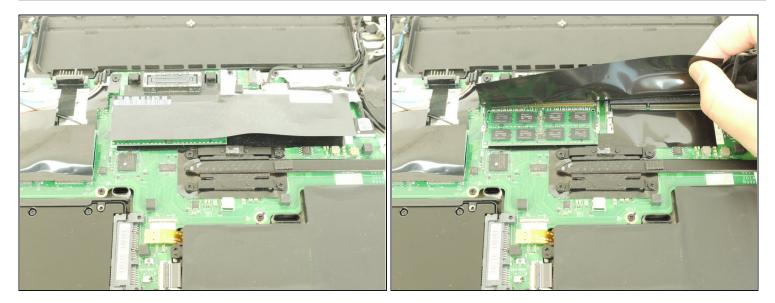
• Lift up the black piece of tape and remove it to uncover the RAM sticks underneath.
