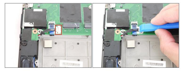
• Disconnect the speaker cable from the motherboard using the plastic opening tool.
