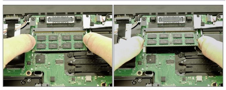
• Using your fingers, push the two clips securing the RAM away from each other to release the RAM.
