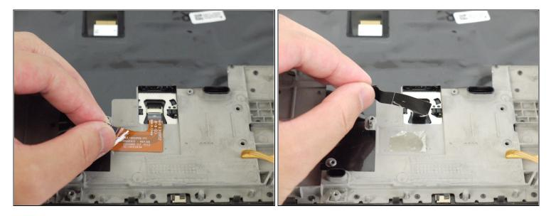
• Using your fingers, carefully peel off the trackpad cable from the device.
