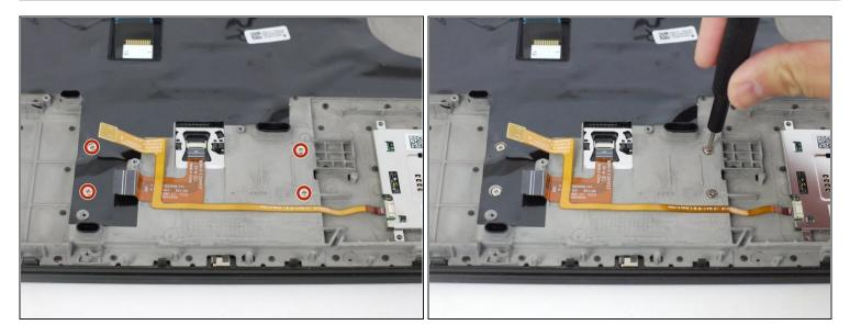
• Using the JIS #00 screwdriver, remove four 3 mm screws securing the trackpad to the device.
