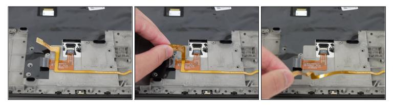
• Using your fingers, grab the smartcard reader cable and peel it off of the device.
