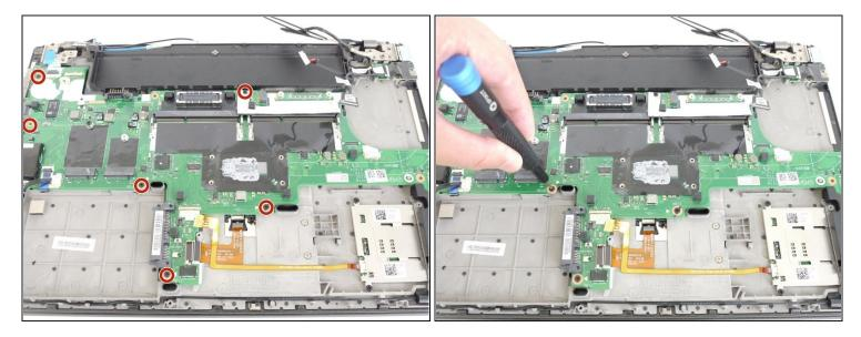
Using the JIS #00 screwdriver, remove six 2.8 mm screws securing the motherboard to the device.
