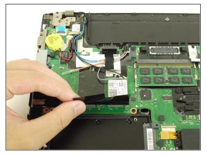
• Lift and remove the black piece of plastic to expose the Wi-Fi card.
