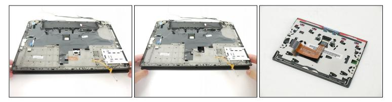
• Lift the bottom panel and remove the trackpad from the device.
