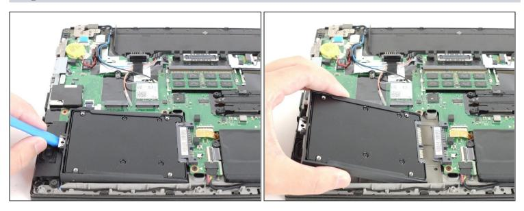
• Lift the SSD up and to the left and remove it from the device.
