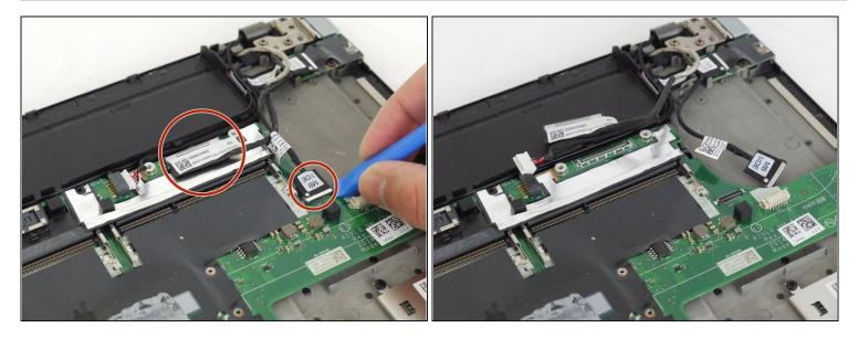
Disconnect the daughterboard cable and the display cable using the plastic opening tool.
