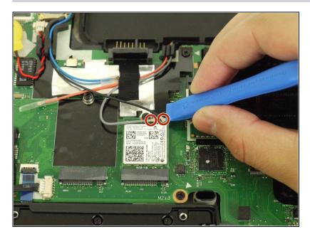
Using the plastic opening tool, disconnect the two cables from the Wi-Fi card.
