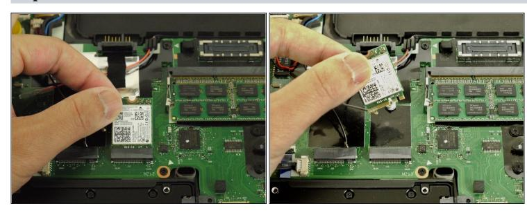
• Lift the Wi-Fi card out of the slot and remove it from the device.
