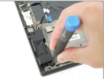
• Using the JIS #00 screwdriver, remove the two 4.2 mm screws securing the left-side speaker to the device.
