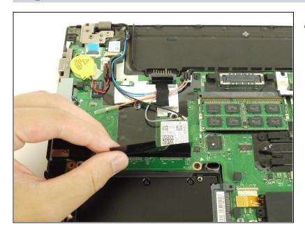
Lift and remove the black piece of plastic to expose the Wi-Fi card.
