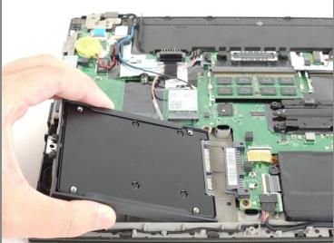
• Lift the SSD up and to the left and remove it from the device.
