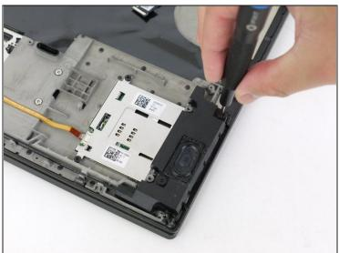
• Use the same JIS #00 screwdriver to remove two 4.2 mm screws from the right-side speaker.
