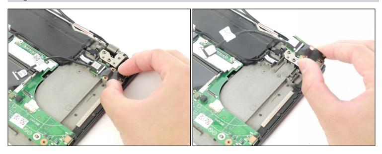
• Lift up and remove the daughterboard from the device.
