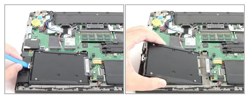
• Lift the SSD up and to the left and remove it from the device.
