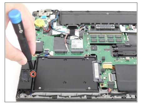
Using the JIS #00 screwdriver, remove the single 2.8 mm screw securing the SSD to the device.
