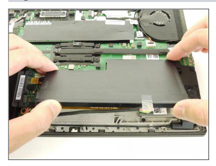
• Lift up and remove the battery from the device.
