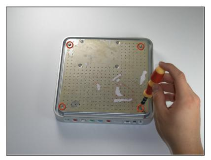
Remove the four T10 Torx screws that secure the lower case to the upper case.
