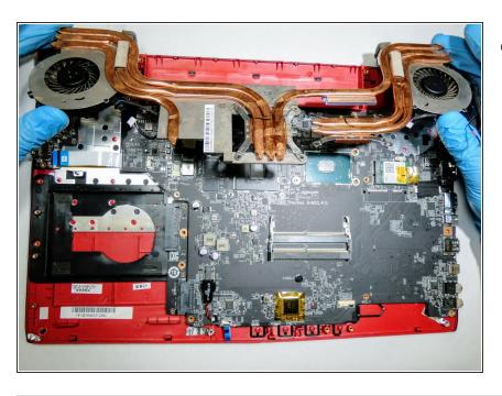
Remove the heatsink from the device.
