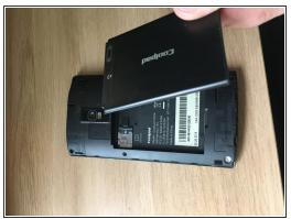
Place a fingernail in the notch at the bottom of the battery. Lift the bottom of the battery up, then
