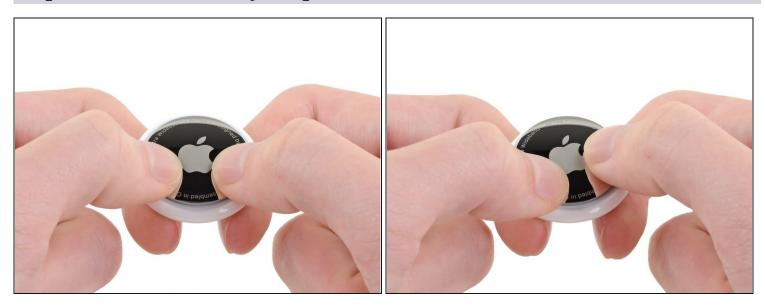
• Rotate the battery compartment door counter-clockwise to unlatch it from the frame.
