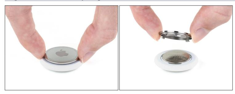
• Lift up the battery compartment door to remove it.
