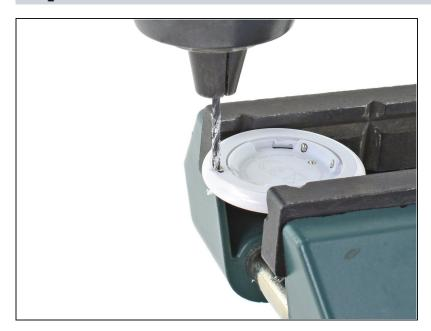
Use a 1/16th inch drill bit to drill a hole through the AirTag.
