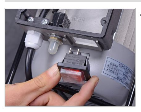
Remove the on/off switch.
