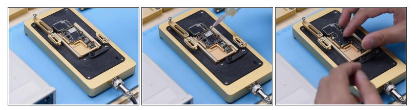
Put the signal board on the Heating Platform. Set the temperature to 180°C to heat. After the solder balls are formed, turn off the power and cool the signal board. Apply some Paste Flux. Align the logic board with the signal board. Keep heating the motherboard at 180 °C.
