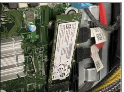
Use the Phillips #1 screwdriver to remove the 3.7 mm screw and remove the old M2 SSD.
