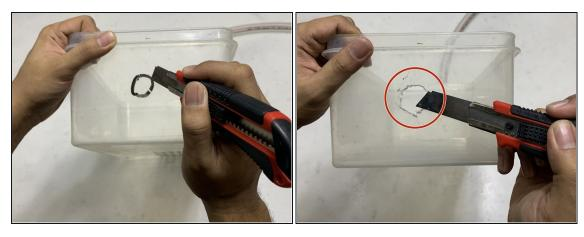
• Use the utility knife to cut a hole in the marked position to attach the pipe.
