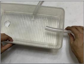
• Insert the soft PVC pipe in the plastic box.
