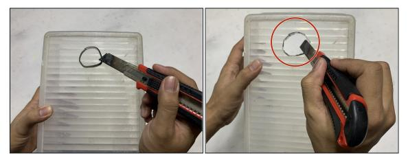
• Using the same utility knife, make a hole in the bottom of the plastic box for the water to come out.
