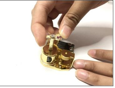
Slowly turn the winding key in the opposite direction to release the tension built-up in the spring.
