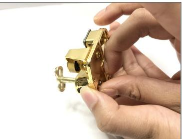
Tap the base of the mechanism a few times to release the governor assembly.
