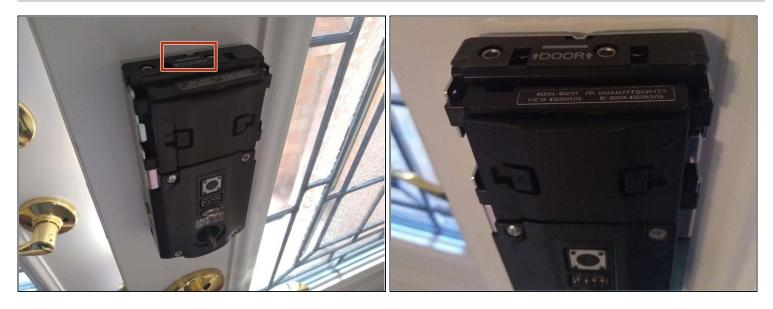
• Find the battery pack (marked "DOOR" in between two arrows) at the top of the lock.
