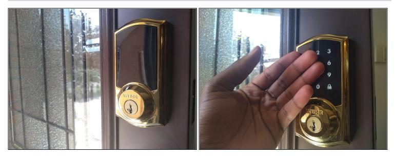
To confirm the finished repair, go to the front of the door and place the back of your hand on the touchscreen to activate the keypad.
