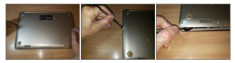
• Insert the spudger into the side of the laptop and slide the spudger around the edges of the laptop to free the back cover from the rest of the device.
