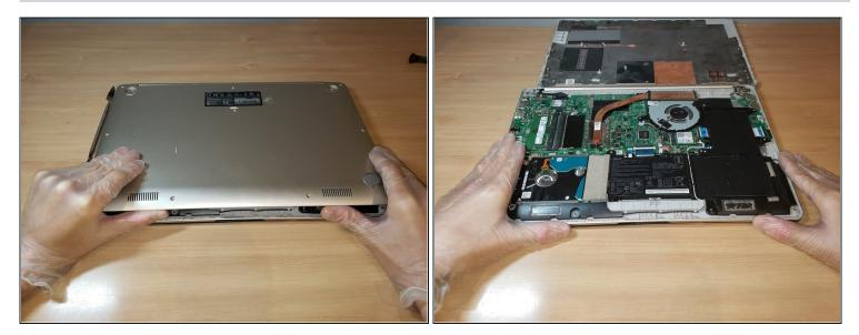
• Remove the back cover from the device.
