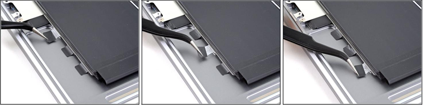
ⓘ The MacBook's battery cells are attached to a metal tray as a complete assembly, which is adhered to the case with a total of six stretch-release adhesive strips.
