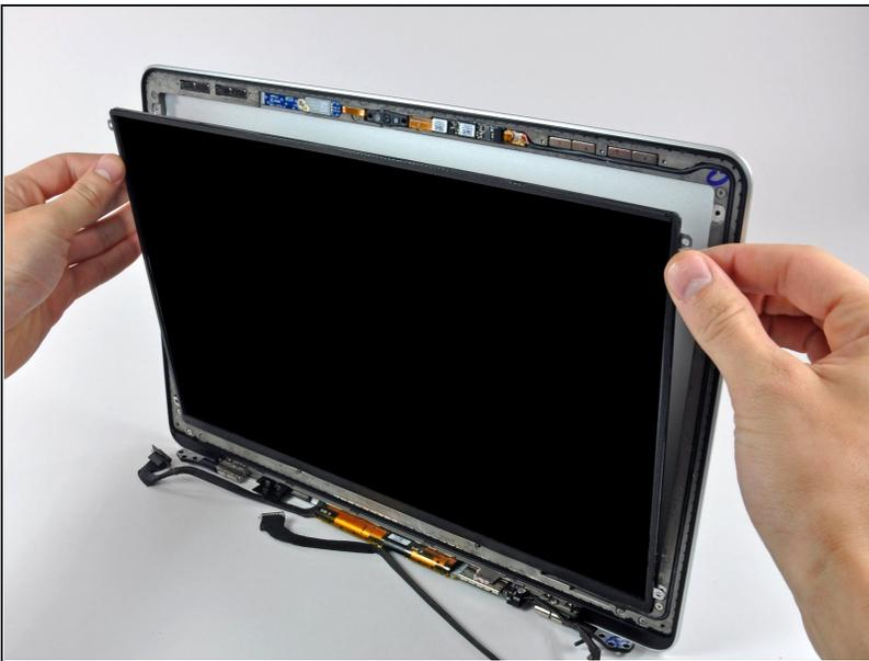
**⚠ Do not try to remove the LCD yet. The circuitry along its lower edge is wedged in a gap along the lower edge of the display recess in the aluminum display assembly.**
