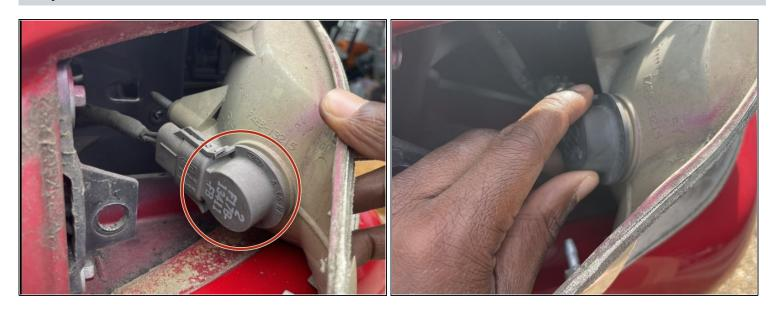
• Take out the turn signal light by twisting it. Remove the side panel.
