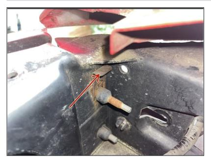
In the same area where you removed the screw, remove the clip by hand or use needle nose pliers.
