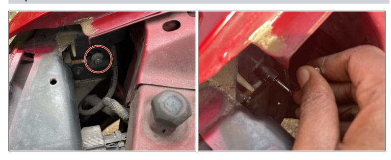
• Using the 11mm wrench, remove the nut.
