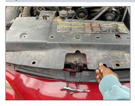
Pull on the edges until the cover pops off revealing the nut shown in the next step.
