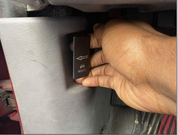
To open the hood, pull the release lever by your foot break inside the car.
