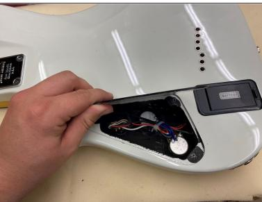
Remove the large plastic backing plate.
