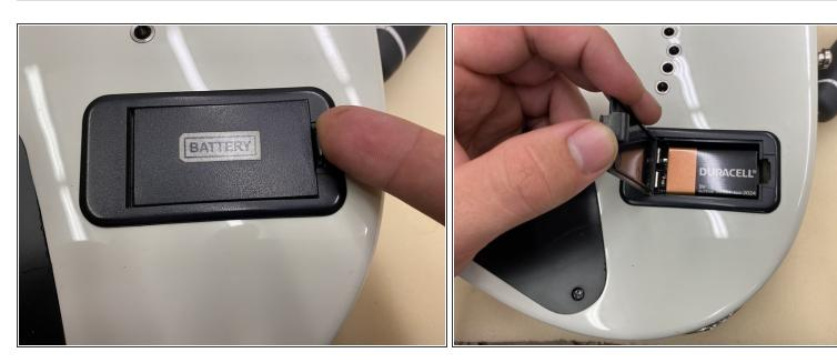
• If the guitar has active pickups, open the battery tray and remove the 9-volt battery.
