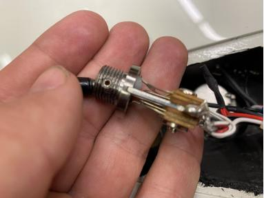
Carefully pull the pickup selector switch out of the body of the guitar.
