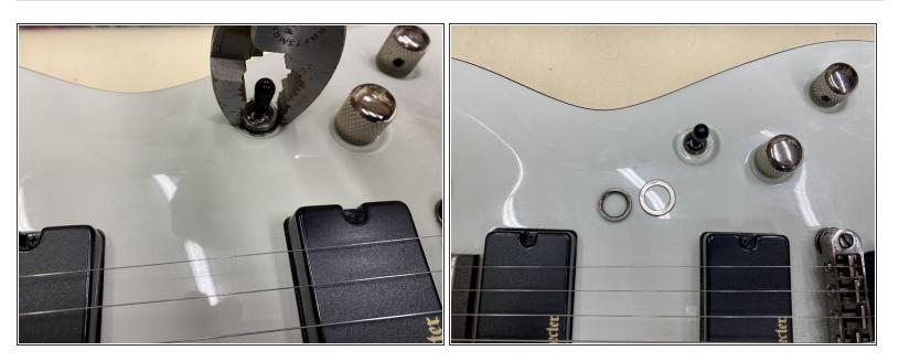
Remove the retaining nut that holds the pickup selector switch to the guitar.
