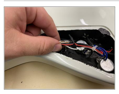
Insert the switch back into the guitar, ensure that the switch is in the correct orientation.
