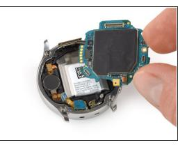
Slide the motherboard out from under the plastic tab to remove it.
