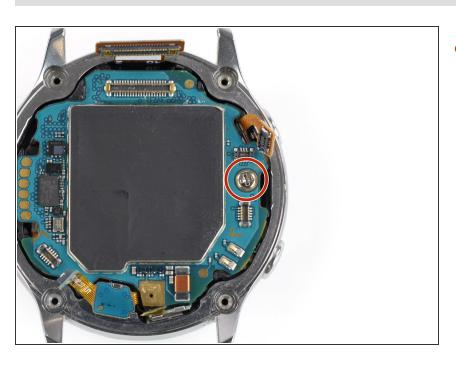
Use a Phillips screwdriver to remove the 4.4 mm-long screw holding the motherboard in place.
