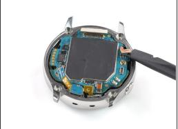
• Use the flat end of a spudger to disconnect the display assembly, the microphone and pressure sensor array, and side button.
