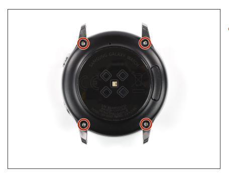
Use a Tri-point Y00 screwdriver to remove the four 4 mm-long screws on the back of the watch.
