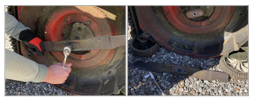
• Use a 5/8 ratchet or wrench to remove the bolt. Then remove the blade.
