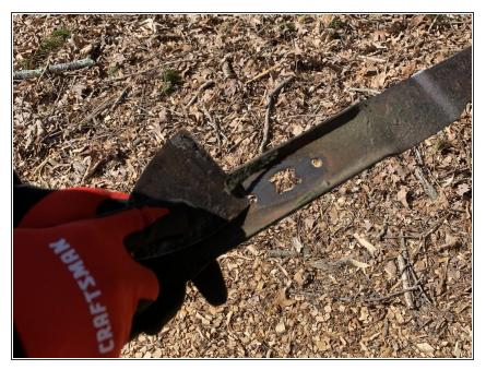
• Clean the blade with a scraper or a wire brush to remove grass residue .
