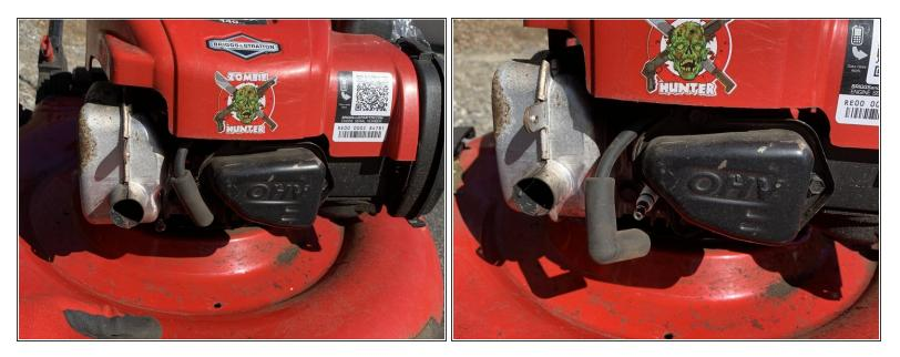
• Disconnect the spark plug wire.
