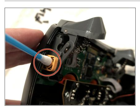
Dip your Q-tip in a bit of isopropyl alcohol and dab a little bit into the arm pot. Be careful not to let any leak over any other parts of the controller.
