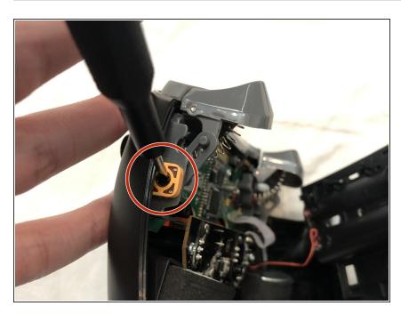
Make minor adjustments to the screw inside the arm pot using your flathead screwdriver.
