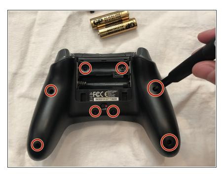
Remove the eight 1 mm screws from the bottom of the controller using the Y1 Tri-Point screwdriver.
