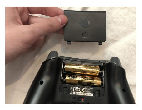
Remove the battery cover and the batteries from the controller.
